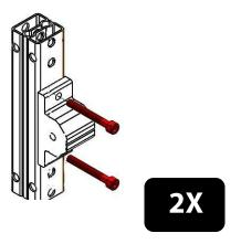
**Step 4**: Take assembled 5.08" Peanut pieces and bolt them onto the two 12" Peanut pieces without holes. Use ½-20 x 2500 Thread Forming Screw (am-1222).
