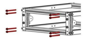
**Step 8**: Attach the ToughBox Micros with 1/4-20x1000 Thread forming screws (am- 1182). Do this to both sides of the chassis.
