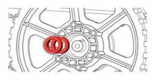
**Step 15**: On both sides push 3/8-16 x 4.25 bolt (am-1297) through the DuraOmni (am-3291), then through a 3/16" thick nylon spacer (am-1181). Push the bolt through the pillow block.
