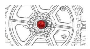
**Step 16**: On the other side put a 3/16" thick nylon spacer and then thread 3/8-16 Nylock Nut (am-1054). Tighten this all the way then back off a half of turn.
