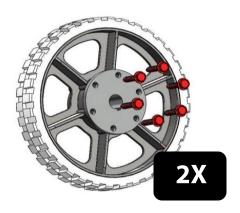
**Step 13**: Slide two 3/16" Thick Nylon Spacer (am- 1181) on each shaft.
