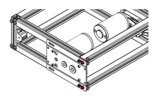
**Step 10**: On each of the ToughBox slide on a 3/16" thick spacer (am-1181). Then slide in a 1/8x1/8x0700 Machine key (am- 1043)
