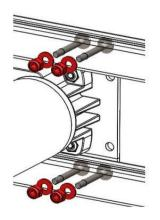
**Step 6**: Take U-Shaped assembly from Step 5 and attach it to the assembly from Step 4 with 1/4-20 Thread Forming Screw (am-1222)
