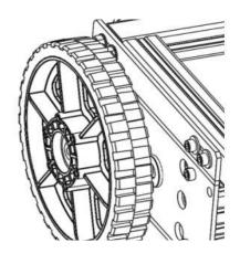
**Step 14**: The end of the ToughBox shaft is threaded inside, insert the ¼-20 x ½ screw (am-1039) through the 1/4" Washer (am-1027) and into the end of the output shaft. This will keep the wheel secure.
