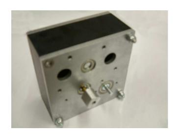
Step 21: Mount the encoder bracket onto the motor plate by using 10-32 x ½" screws. Press the encoder disk onto the shaft over the encoder so that the outer face of the encoder disk is flush with the tips of the encoder mount clips. Press the encoder cap over the encoder.
