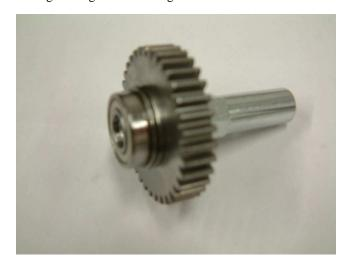
Step 7: Attach the dog gear to the shift block and assembly with loctite in the 2.5mm screw.
