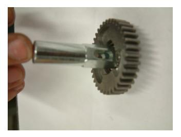
Step 6: Insert the shift block through the small brass spacer and shaft assembly into the SS hex shaft hole.
