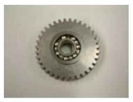
Step 4: Insert the gear over the small end of the Super Shifter hex shaft.
