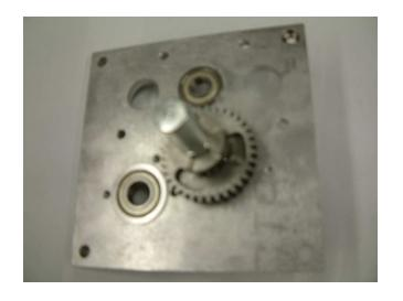
Step 5: Place an FR6ZZ bearing over the shaft, with the flange facing the 35-tooth gear.
