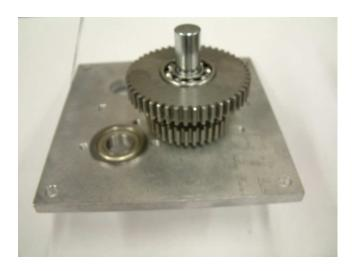
Step 12: Slide the 40T gear, the 15T gear, and the brass spacer onto the backside of the 28T gear.
