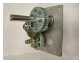
Step 18: Grease the gears and place the SS housing over the motor plate. Slide the output plate over the shaft.
