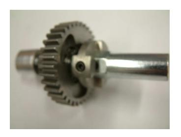
Step 9: Press an R8 bearing into the 48T output gear.
