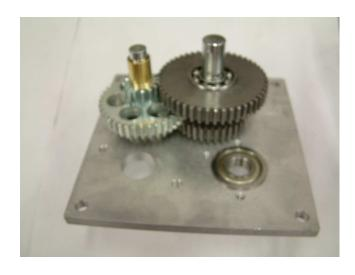
Step 15: Insert the ½" e-Klip onto the SS output shaft. Place the 45T gear on the SS output shaft.
