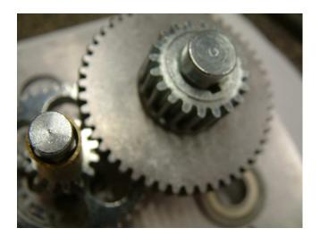
Step 11: Take the SS cluster shaft and place the 22T gear with the boss facing away from the middle.
