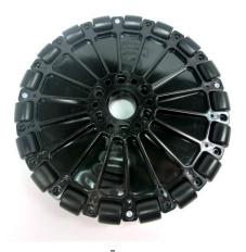
Step 6: Insert a M3 nylock nut and screw it in with its M3 x 10mm SHCS until all holes have been filled.
