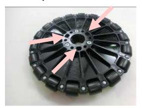
Step 3: Cover the three #10-32 x 2-1/4" SHCS with your hand and turn the wheel over. Screw in the M5 Nylock Nuts by hand.
