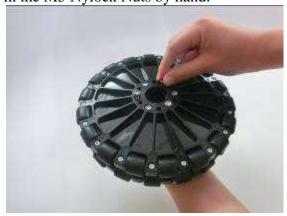
Step 2: Place the other omni wheel above it. Align the holes so that the three #10-32 x 2-1/4" SHCS will go into the holes that have the arrows on them. Insert and tighten in three #10-32 x 2-1/4" SHCS with the cordless drill. Make sure the rollers are alternating.
