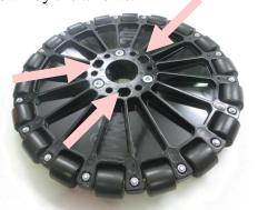
Step 2: Press in an R8 ½" id bearing to the top off the first wheel, and to the bottom of the second omni wheel.
