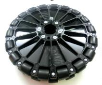
Step 4: Cover the three  $#10-32 \times 2-\frac{1}{4}$ " SHCS with your hand and turn the wheel over. Screw in the M5 Nylock Nuts by hand.
