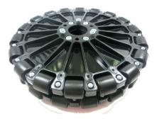
Step 6: Press in a ½" id flanged, shielded ball bearing to each side of the assembled dualie omni wheel.
