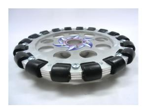
Step 2: Insert and tighten in six #10-32 x  $^{1}/_{2}$ " SHCS with the cordless drill.
