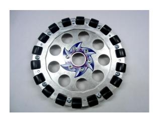
Step 3: Turn it upside down and place the other omni wheel on top of the aluminum spacer. Insert and tighten the remaining six screws into the spacer. Make sure you insert these last six screws into the alternating holes of the spacer. It should look exactly as shown to the right.
