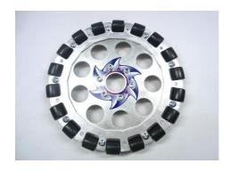
Step 4: With a press, insert the ½" FR8ZZ Bearings on each side of the omni wheel.
