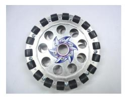
Step 2: Insert and tighten in six #10-32 x  $\frac{1}{2}$ " SHCS with the cordless drill.
