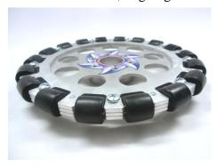
Step 3: Turn it upside down and place the other omni wheel on top of the aluminum spacer. Insert and tighten the remaining six screws into the spacer. Make sure you insert these last six screws into the alternating holes of the spacer. It should look exactly as shown to the right.
