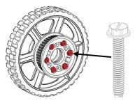
Step 4: Add two more pulley halves (am-2234-half) to the wheel.
