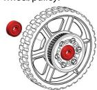
NOTE: Tighten the screws in a triangle pattern to ensure the pulley aligns evenly on the wheel.
