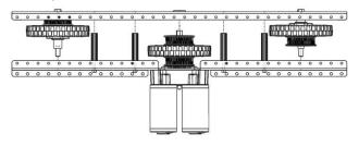
The long chassis requires 160 tooth belts (am-2266). The wide chassis requires 120 tooth belts (am-2704). The square chassis requires 131 tooth belts (am-2571).
