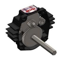
\*To change the drive speed of the AM14U3, different gear ratios can be used in the Toughbox Mini. The AM14U3 features a center wheel directly driven by a TB Mini Hex Output Shaft. To change the ratio and drive speed, the standard 16 tooth Small Cluster Gear and 48 tooth Large Output Gear will need to be replaced with two gears totaling 64 teeth.
