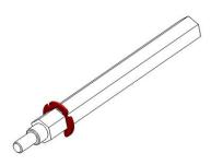
**Step 7:** Place the 48 Tooth Gear (am-0885) on TB Hex Output Shaft **flat side down**.
