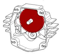
**Step 5:** Tap the 1/2" E-Clip (am-0206) onto the groove on the TB Hex Output Shaft (am-2566).
