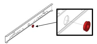
**Step 19**: Add the long spacer (am-1307), Outer Wheel Assembly and the short spacer (am-1306) onto the axle bolt. The shorter 0.28" (am-1306) spacer is used on the pulley side of the wheel.
