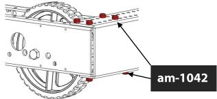
NOTE: The long chassis will use 6 screws and nuts per corner. The wide and square configurations will use 5 screws and nuts per corner.
