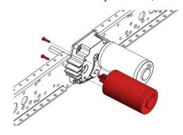
**Step 10:** Place the TB Mini onto the Inner Plate using the plastic studs to align the housing. The bottom flanged edge of the Inner Plate will be facing towards the gearbox housing.
