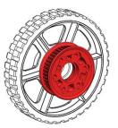
**Step 2:** Using six 10-24 x 1.25" (am-2234-half) to the wheel (am-0940a). 1266) thread forming screws, attach the pulley halves to the wheel.
