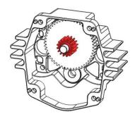
**Step 6:** Insert the small end of the TB Hex Output Shaft (am-2566) into the other R6ZZ bearing.
