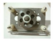
Step 5: Tighten the 10-32 Nylock Nuts on 10-32 Screws.
