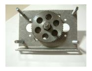
Step 4: Place the second Motor Plate onto of the assembly. Make sure that the curve is on the opposite side of the screws.
