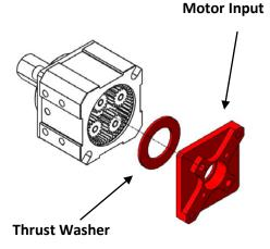
**Step 5**: Be sure to add a pea-sized amount of included Red Tacky Grease (am-2768) to the gear teeth. If more than one stage is present in the gearbox, add grease to each stage.
