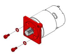
**Step 6**: Reinstall the Thrust Washer into the 57 Sport onto the surface of the gears inside the gearbox. Insert the Motor Assembly into the gearbox, and gently turn the output shaft until the gears mesh.
