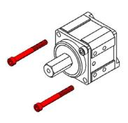
**Step 4**: Attach the Motor Input Block to the RedLine, 700 or 500 series motor (with previously attached pinion) using the included M4-0.7 Socket Head Screws and M4 Lock Washers. Be sure to install the Motor Input Block with the non-circular side against the motor.
