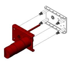
**Step 10**: Secure the gearbox together with four 1/4-20 Nylock Jam Nuts (am-1102)
