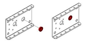
NOTE: Make sure the flange of the bearing is flush against the sheet metal of the gearbox plate.
