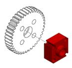
**Step 2**: Use four 6-32 x 0.500" long Button Head Screws (am-1418.) to attach the gear to the nub.
