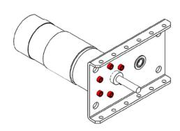
**Step 4**: Install the 6mm D-Shaft (am-3226-100) into the center bearing such that the end of the shaft is
