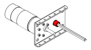
**Step 7**: Install a Gear Assembly onto each of the NeveRest Motor shafts such that all of the gears in the Gear Assemblies are lined up. Tighten the #10-32 Set screws to lock all the gear assemblies in place.
