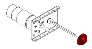
**Step 1**: Press a 6x12x4 Flanged Bearing (am-3377) into the center 12mm hole of a PicoBox Uno gearbox plate (am-3423).
