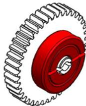
**Step 3:** Make sure the slot on the gear boss lines up with the slot on the collar clamp.
