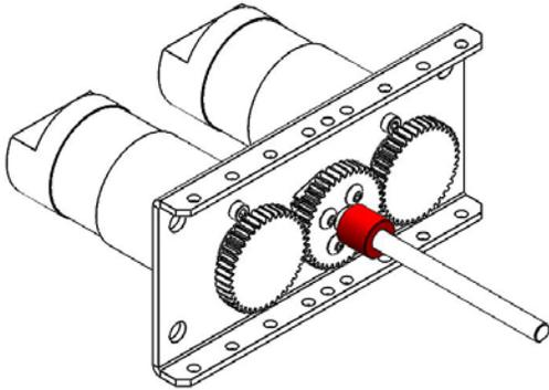
**Step 8:** Press a 6x12x4 Flanged Bearing (am-3377) into the center 12mm hole of a PicoBox Twin Turbo gearbox plate (am-3439).
