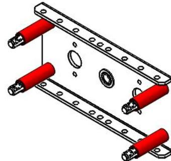
**Step 11:** Insert the Axle of the Gearbox Assembly into the bearing on the PicoBox Twin Turbo gearbox plate. Align the four 1/4-20 screws with the 1/4" holes on the PicoBox Twin Turbo gearbox plate is up against the Picobox Spacers.
