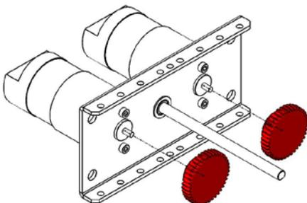
**Step 6:** Install a Gear Assembly onto the axle such that all of the gears in the Gear Assemblies are lined up. Tighten the #10-32 Set screws to lock all the gear assemblies in place.
