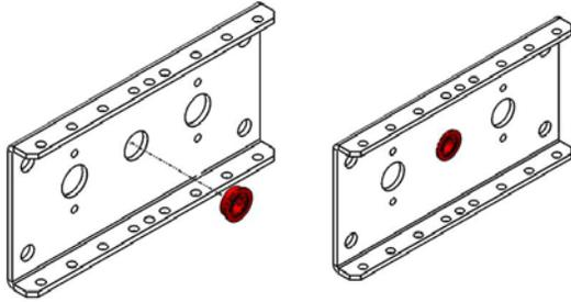
**NOTE:** Make sure the flange of the bearing is flush against the sheet metal of the gearbox plate.
