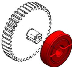
**Step 2:** Be sure to insert the boss of the gear into the cavity of the collar clamp.
