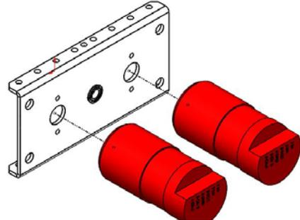
**Step 3:** Install six M3-0.5 x 6mm long socket head screws (am-1254) in each NeveRest motor to secure it to the gearbox plate.
