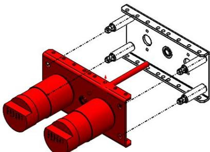
**Step 12:** Secure with four 1/4-20 Nylock Jam Nuts (am-1102)
