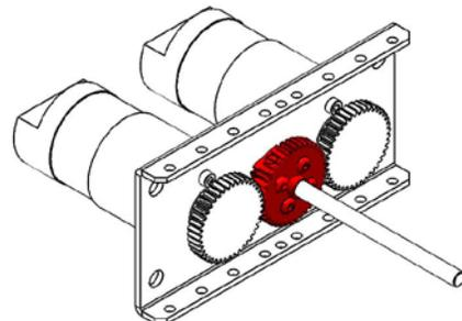
**Step 7:** Install the Aluminum Spacer (am-3481) on the center axle up against the previously installed bearing.
