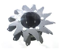
Step 3: Turn it over. Place the inner 10" mecanum steel plate above the wheel, aligning the M6 x 1.0 x 120mm Hex Head Screws with the holes.
