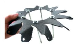
Step 2: Insert this assembly into the 10" Mecanum Hub. Hammer in the screws.
