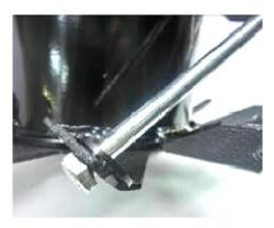
Step 8: With the cordless drill and socket, tighten a M6 x 1.0 Nylock Nut to the M6 x 1.0 x 120mm Hex Head Screw.
