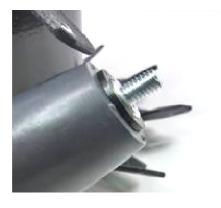
Step 6: Insert a M6 x 1.0 x 120mm Hex Head Screw along with a ½" i.d. Plastic Washer into one of the 10" steel mecanum plates.
