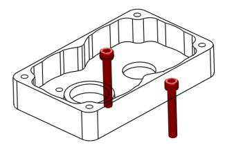
**Step 2:** Slide the CIM Spacer (am-0555) in place through the screws.
