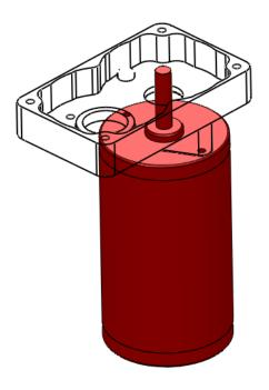
Step 4: Place the 0.475" Long Nylon Spacer (am-0925) onto the CIM Motor shaft followed by the 0.375" Long Spacer
