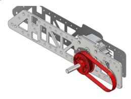
**Step 5**: Mount six churros (am-2569) to the Inside Plate, sticking out the same side as the gearbox output shaft, each with a 1/4-20 screw (am-1310). Mount Outside Plate to the six churros (am-2569), aligning the Outside and Inside Plate edges with the 1/4-20 thread forming screws (am-1310). Churros do not need to be pre-tapped.
