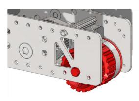
Step 10: Install middle Pulley Wheel by inserting 3/8 axle bolt (am-1297) into the middle of Main Body, through Outside Plate, 3/8" washer (am-1393), Pulley Wheel, gray plastic spacer (am-0441), and Inside Plate. Thread the 3/8-16 nut (am-1394) on end of 3/8" bolt, tightening until Pulley Wheel does not spin. Loosen this nut 1/2 turn so the Pulley Wheel spins freely.
