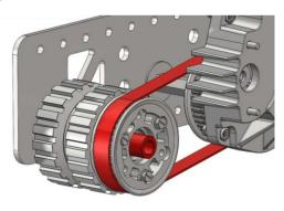
Step 9: Move the pulley into position at the 3/8" axle hole at the back of the Main Body. Insert the 3/8 axle bolt (am-1297) into 3/8 hole of Main Body, through Outside Plate, 3/8" washer (am-1393), Pulley Wheel, gray plastic spacer (am-0441), and Inside Plate. Be sure the 85 tooth timing belt is in position as this wheel is installed. Thread the 3/8-16 nut (am-1394) on 3/8" bolt, tightening until Pulley Wheel does not spin. Loosen this nut 1/2 turn so the Pulley Wheel spin freely.
