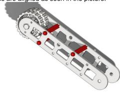
Step 14: Adjust the turnbuckle (am-3321) to be short. Insert 3/8" bolts for turnbuckle mounting through non-used 3/8" holes, one on Upper Arm and one on Main Body. Install 3/8" collar clamps (am-2382), turnbuckle eye, white spacer (am-0243), and 3/8" washers (next to turnbuckle) on axle. Install 3/8-16 Nuts onto turnbuckle bolts and tighten. Position collar clamps (am-2382) on outside of eye bolt portion of turnbuckle and tighten collar clamps.
