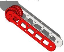
Step 13: Position Upper Arm assembly onto Main Body assembly so Upper Plates are outside of the Main Body plates, the 3/8" holes are aligned, and the Upper Arm is positioned as shown. Insert the 3/8" axle bolt (am-1297) into the 3/8" holes at this hinge, through these parts: Upper Plate, Outside Plate, 3/8" washer (am-1393), Pulley Wheel, brass spacer (am-2243), 3/8" washer (am-1393), Upper Plate, Inside Plate. Tighten the 3/8 nut (am-1394) on axle bolt. Back off the nut 1/2 turn.
