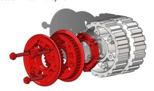
**Step 8**: Install back Pulley Wheel assembly (with the 42 tooth pulley assembled) by placing the gray plastic spacer (am-0441) inside the 42 tooth pulley and wrapping the 85 tooth belt (am-2703) around the 42 tooth pulley. (picture below shown without Inside Plate)
