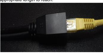
Step 4: Connect the previously mentioned Ethernet cable to radio. Be sure to plug the Ethernet cable into the plug nearest the power barrel.
