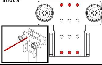
**Step 2**: Use a Try Square to ensure the bottom of the Corner Bearing Assembly is perpendicular with the 1" wide faces of the Carriage Vertical Tube. Align the inside surface of the notch (as shown with arrows,) with the outside surfaces of the Tube.
