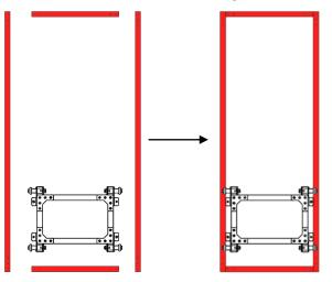
**Step 3**: Align a 90 degree gusset to the outer edges of one corner of the Frame as shown.
