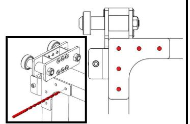
**<u>Step 16</u>**: Repeat Steps 13-15 for the remaining **seven** gussets to finish assembling the Carriage as shown.
