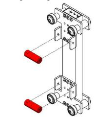
**<u>Step 6</u>**: Rivet the Small Bearing Plate in place with six 3/16" x 1/4" Steel Rivets.
