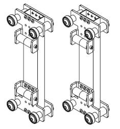
**<u>Step 13</u>**: Align a 90 degree gusset (am-3860) with both tubes as shown.
