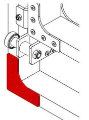
**<u>Step 5</u>**: Rivet the gusset in place with five 3/16" x 1/4" Steel Rivets.
