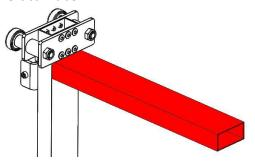
**Step 14**: Match drill the rivet holes through the gusset to the nearest side of each tube in the locations shown with a red dot.
