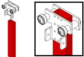
**Step 3**: Match drill the rivet holes with a #9 (0.196") drill bit through the Large Bearing Plate into the nearest side of the Tube in the locations shown with a red dot.
