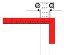
**<u>Step 4</u>**: Rivet the Large Bearing Plate in place with six 3/16" x 1/4" Steel Rivets (am-1226)
