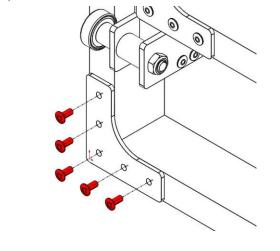
**Step 2**: Carefully clamp the Frame together between the arrows, and ensure it slides freely. Check the left/right movement of the carriage. If it exceeds 1/32", the Frame Horizontal Tubes should be trimmed to avoid potential binding.
