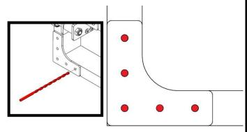
**<u>Step 6</u>**: Repeat Steps 3-5 for the remaining **seven** gussets to complete the Frame as shown.
