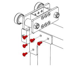
**Step 12**: Place a Carriage Horizontal Tube against the 2" face of the Carriage Vertical tube, and the bottom of Small Bearing Plate. Line up the 1" wide face of the Carriage Vertical Tube to the 1" wide face of the Carriage Vertical Tube.
