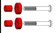
**Step 2:** Slide one Large Bearing Plate (am-3794a) and two 1" Long Aluminum Spacers (am-1450) onto the two 3/8" x 2.75" BHCS.
