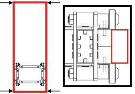
**Step 4**: Match drill the rivet holes through the gusset to the nearest side of each tube in the locations shown with a red dot.
