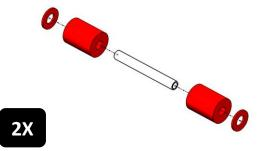
**Step 10**: Secure each roller assembly with a #10-32x2.75" SHCS (am-1397) and a #10-32 Nylock nut. (am-1042) **Do not over-tighten the screws.**
