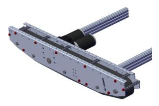
**Step 31:** Connect the other Inside Plate (am-4011) to the other side of the Walnut Extrusions using ¼-20 x .0750 Thread Forming Screws. Ensure the bottom flanges of each Inside Plate are pointing toward each other and ensure the bottom screws in the rear Walnut Extrusion are left out.
