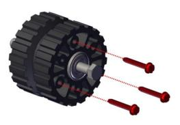
**Step 5**: Add one 250 Pulley and Sprocket Spacer (am-0207a) and a 22T #35 Sprocket (am-0216) to the pulley assembly. Secure using three 10-24 x 0.750 thread forming screws (am-1123).
