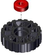
**Step 2**: Combine two pulley/bearing assemblies together, and temporarily insert a \%-16 x 4.25 Bolt (am-1297) through the pulley assembly to keep the bearings aligned.
