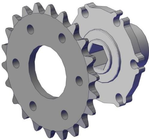
**Step 2:** Insert six 10-32 x 0.750 SHCS (am-1047) screws through the plate sprocket into the holes in the hub. Secure with six 10-32 Nylock Nuts (am-1042). Be sure to tighten in a star pattern to maintain alignment.
