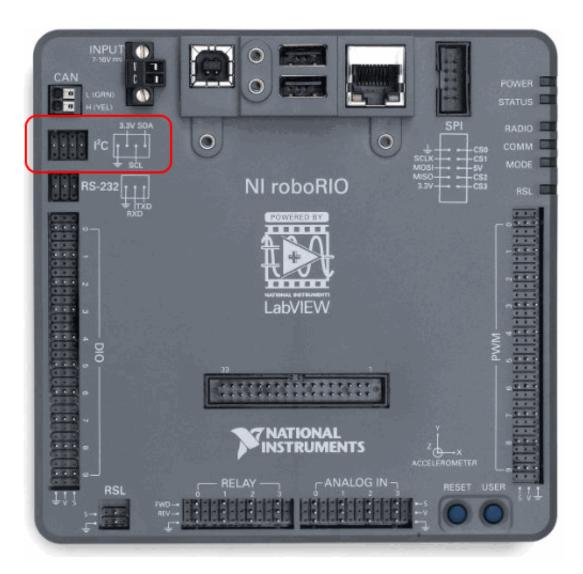
IMPORTANT NOTE: The left-to-right order of the RoboRIO Onboard I2C Interface Pins is different than the navX-Micro I2C pin left-to-right order.
