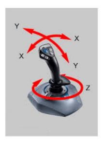
Since a three-axis joystick is typically used to control a robot, the robot designer must select upon which Reference Frame the driver joystick is based. This selection of Reference Frame typically depends upon the drive mode used:
