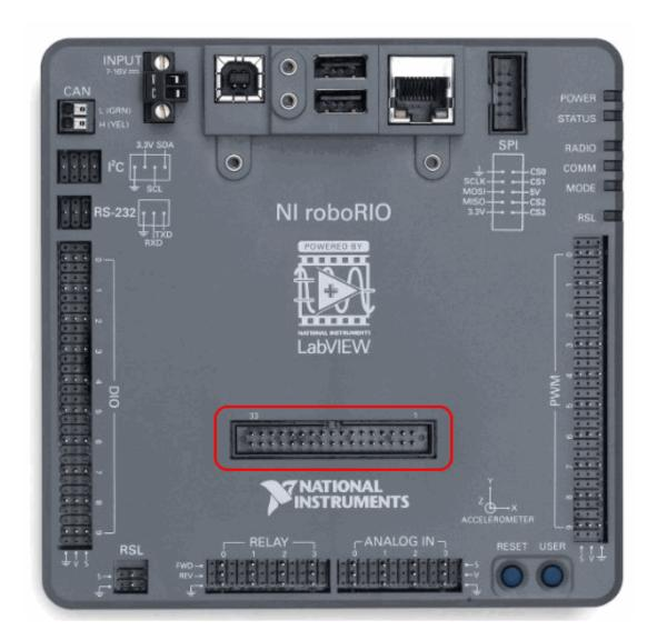
As shown in the diagram below, the RoboRIO MXP Connector's I2C-related pins are:
