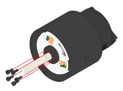
Step 5: Remove the Shaft
