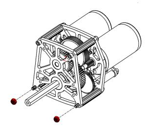
**Step 5**: Flip the Inside Plate over, and install two #10-32x0.750" SHCS through the Inside Plate into the EVO Shifter. Also, install one 500Hex x 0.25" Spacer (am-3948-250) against the hex bearing in
