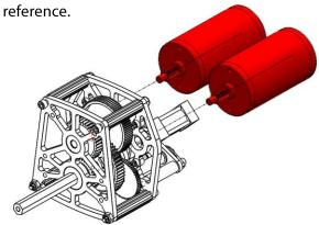
**Step 4**: Line up the bottom two screws with the large holes on the Inside Plate of the AM14U4 on the same side as the bottom flange. Insert the hex shaft into the large bearing hole, as well as the screws into the 1/4" diameter holes. Reinstall the nuts removed in Step 3, but do not fully tighten.
