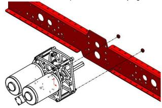
**Step 6**: Secure the #10-32 screws with #10-32 Nylock Nuts as shown. Tighten the bottom 1/4-20 Nylock Nuts.
