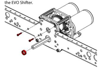
**Step 2**: Install the CIM Motors with pinions into the EVO Shifter using the included #10-32 x 0.625 SHCS with Nylon Patch. A 2 Stage EVO Shifter is shown for
