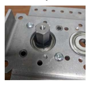
**Step 5b**: Place two #10 fender washers on the top of the shaft and secure the stack in place with a 3/8 in. long #10-32 thread patch button head cap screw.
