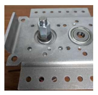
Step 2a: Place the 8mm key to 1/2 in. hex adapter over the shaft and place the spacer plate on the face of the motor with the holes aligned. Note: This spacer is only needed if all 4 washers were used in step 1a. It is needed to let the CIM clear the bearing in the next step.
