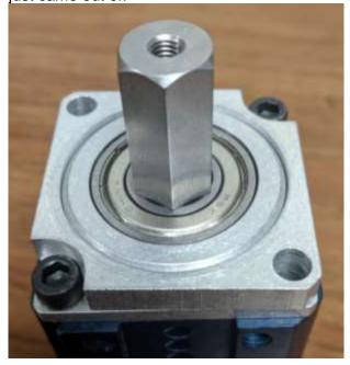
**Step 2b:** Install the 3/8 in. ID bearing in the bearing hole in the plate furthest from the bent tab. The flange of the bearing should be on the same side as the tab. Place this assembly on top of the Sport gearbox as shown.
