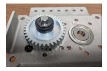
**Step 1b:** Section "b" covers preparing a 57 Sport, or similar, gearbox with a 1/2 in. hex output shaft to be the input to the Flyer. If using a Falcon 500 Please skip ahead, if using a CIM style motor go back to section "a".
