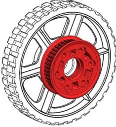
**Step 2:** Using six 10-24 x 1.25" (am-1266) thread forming screws, attach the pulley halves to the wheel.
