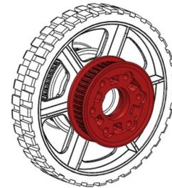
**Step 5:** Insert one 500EX Hex Hub (am-2568) into the pulley on one side of the wheel.
