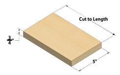
For the corner bumper configuration, 8 planks are needed for each red set and blue set of bumpers. Longer sections are needed to get more coverage on the robot.
