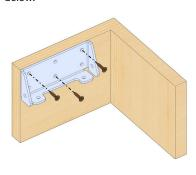
**Step 6:** For corner bumpers, align Side Bracket (am-3962) to the edge of the bumper plank.
