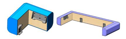
**Step 10:** Attach bumpers as shown with  $10-32 \times 3.75$ " round head screws (am-1502) and 10-32 wing nuts. (am-1387) for easy installation and removal.
