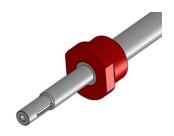
**Step 4:** Apply thread lock adhesive on the Brass Nut and Ram Cap outer threads. Hold the flats of the Ram Cap in a vice with a rag to protect marring on the Ram Cap. Screw the Ram Cap onto the Ram Tube while also threading it onto the Brass Nut. Use a ¾ wrench to tighten the Rap Cap.
