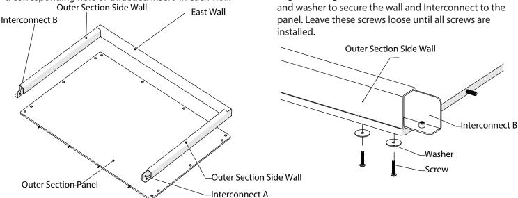
3. Add a screw, washer and spacer to each of the remaining panel holes. Thread the screw into the threaded insert and leave loose until all the screws are installed.
