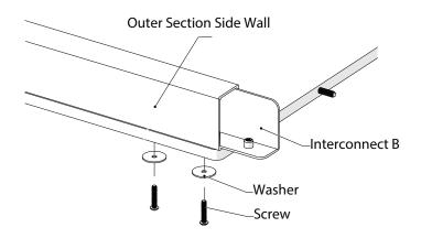
3. Add a screw, washer and spacer to each of the remaining panel holes. Thread the screw into the threaded inserts in each side wall and **leave loose** until all the screws are installed.
