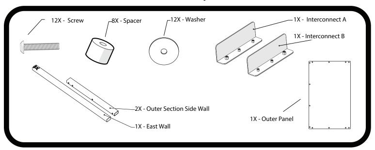
1. Align walls to edges of panel with the flat side of the panel facing up. Each hole in the panel should line up with a corresponding hole or thraeded insert in each wall.
