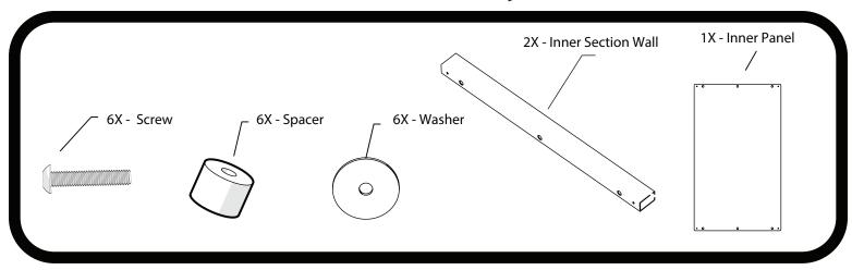
1. Align walls to edges of the inner panel with the flat side of the panel facing up. Each hole in the panel should line up with a corresponding hole or threaded insert in each wall.
