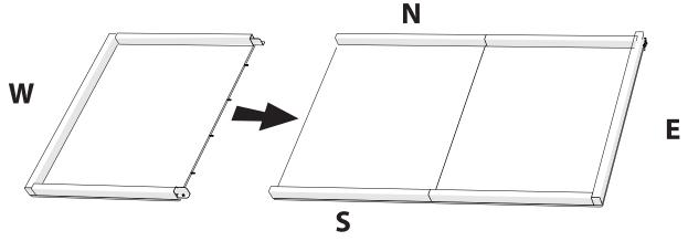
2. Secure sections together using 4X Flat Head Screws. These screws will fit in the countersunk holes on the four corners of the inner panel.
