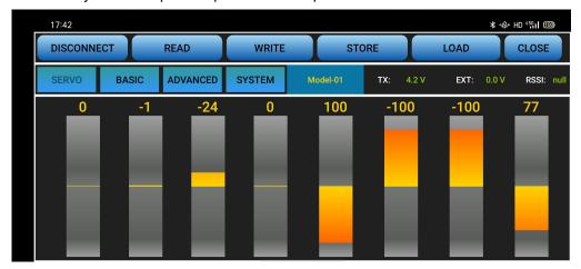
(DIS)CONNECT: When APP is opened on the mobile and T8S is powered on, click CONNECT and a list of Bluetooth devices will pop out and select the RadioLink device to make connection. The two leds at the rightmost will flash in turn with DD sounds, press any of the trimmer buttons to stop the DD sounds and the servo range will display on the APP. If fails, press DISCONNECT and CONNECT again.
