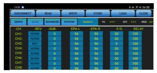
**REV:** Defines the relationship between the transmitter controls and the receiver output for channels with options of NORM and REV. Make sure to check all servos move to the correct direction as wish under control. Make sure to check all servos move to the correct direction under control.
