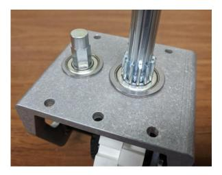
**Step 3d**: Place the previously assembled am-3009\_center onto the two protruding shafts as shown.
