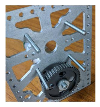
**Step 7d**: Place the motor on the opposite side of the plate and install using the BHCS.
