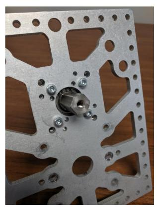
**Step 4c**: Slip the 1/2: in. hex gear (am-4056) over the hex shaft and install the 10-32 SHCS (am-1120) and the fender washer (am-1523) to the end of the PG hex shaft to retain the gear.
