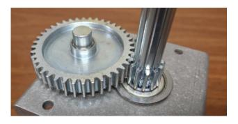
**Step 4d:** Locate four 5/8 in. long aluminum spacers (am-2919a), four 1.25 in. long #10-32 screws, and four nylock nuts. Install these in sets around the top of the yoke to join the bearing plate to the yoke.
