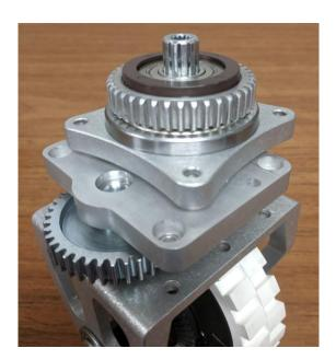
**Step 2d:** Place the 3/8 in. hex bore gear (am-3976) on protruding hex shaft so that it meshes with the drive shaft gear.
