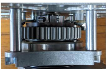
**Step 14d:** (As you continue pressing, make sure that the 4 screws with spacers align to the 4 holes in the bearing plate.
