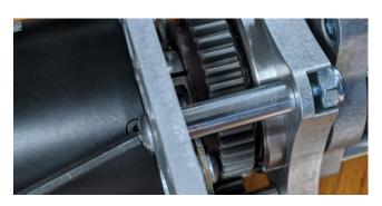
If using a NEO one of the screws will be under the motor wires, but can be accessed by carefully parting the red and black wires. A ball-end Allen wrench is recommended here.
