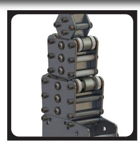
"Spring out, winch back" powertrain is accomplished by using constant force springs and robust Dyneema Rope to retract.
