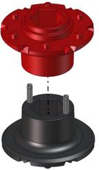
**Step 2:** Press the two 3/32 in. Diameter x 5/8 in. Long Steel Slotted Spring Pins (am-1597) into the two small holes surrounding the hex bore.
