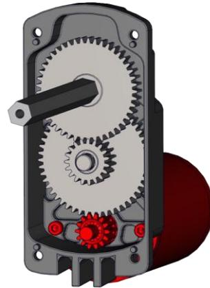
**Step 9:** It is generally recommended to run in the gearbox for a period of time prior to greasing. Grease all gears.
