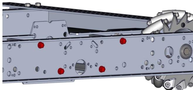
**Step 4:** Grab a Left Wheel Assembly and repeat steps one through three, for the second output shaft on the same side of the frame.
