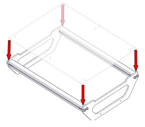
**<u>Step 6</u>**: Wrap the 6 cable ties (am-1189\_1) through the pre-drilled holes in the Driver Tray Bottom Panel and around the Peanut Extrusion. Tighten until fully secure.
