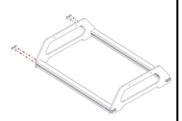
**<u>Step 4</u>**: Place the Driver Tray Bottom Panel (am-4548\_panel) onto the Peanut between the handles.
