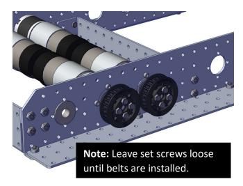
**Step 9**: Install two % Flanged Hex Bearings (am-4489) in the MecanAM Side Plate with the bearing flanges on the same side as the flange on the side plate.
