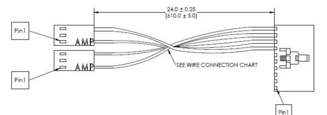
FIGURE 10 - CONTROL MATING CONNECTOR (C2)
