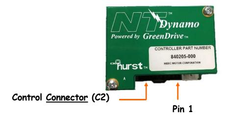
Connect the control inputs and outputs to the GreenDrive<sub>TM</sub> using a 10-pin connector (Molex P/N 50-57-9410 or equivalent) and terminals (Molex P/N 16-02-0103 or equivalent).
