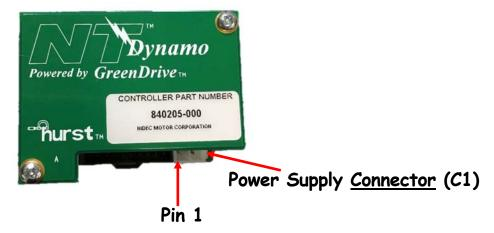
Connect the power supply to the GreenDrivetm using a 2-pin connector (Molex P/N 39-01-2020 or equivalent) and terminals (Molex P/N 39-00-0039 or equivalent).
