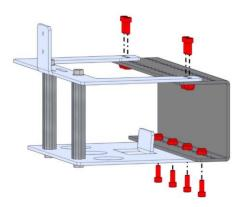
**Step 5:** Secure the Robot Side SB-Series Battery Connector to the tab on the C Plate using two #6-32 x 0.750" Hex Head Screws (am-1424) and #6-32 Nylock Jam Nuts (am-1419). The wires from this connector should go to your main robot breaker and power distribution panel.
