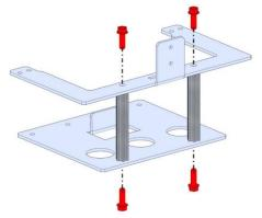
**Step 2:** Slide the assembly over the End Plate. The C Plate and Bottom Plate should be installed on the top and bottom of the flanges on the End Plate, respectively.
