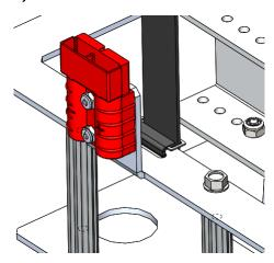
**Step 8:** Plug the SB connector from the battery into the SB connector mounted to the tray. Secure with a cable tie around both connectors through the small slot in the C Plate to ensure the battery will stay connected during match play.
