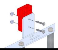
**Note:** The screws should be oriented such that the heads of the screws are on the Tab side.
