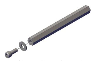
9. Add a 1/4 inch shaft spacer (am-1698) and insert shaft assembly through the two 14T pulley halves and through the previously installed bushings in the tube.
