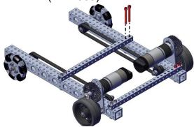
**Note:** Attach the tubes to the center hole pair and the second hole pair on the motor side.
