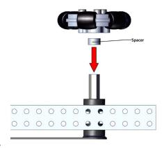
17. Retain wheel with one  $10-32 \times 0500$  inch screw (am-1002) with one #10 washer (am-1026).
