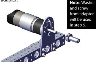
2. Install one NeveRest Orbital 19.2 gearmotor (am-3637b) to the Motor Mount plate using three M3-0.5 8mm patched screws (am-1500) in the lower three mounting holes.
