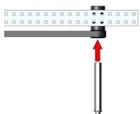
16. Slide one ¼ inch shaft spacer (am-1698) on the shaft from the outside and follow it with one 3 inch omni wheel (am-4967).
