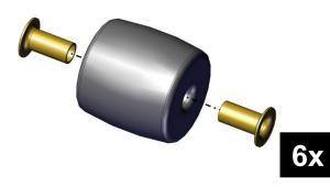
3. Stack an inner plate (am-4967\_inner) and an outer plate (am-4967\_outer) and place a roller assembly in between each spoke.
