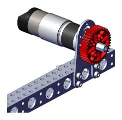
5. Place a ½ inch shaft spacer (am-1699) on the adapter shaft and retain with the washer and screw provided with the adapter.
