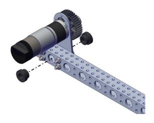
8. Put together two pulley halves (am-4960 half) to create a pulley.
