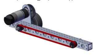
15. Insert the 3 inch shaft assembly through 14T pulley and previously installed bushings.
