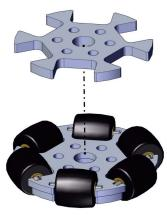
5. Fasten the stack to a hub (am-4967\_hub) with three 10-32 x 0750 inch screws (am-1047) in alternating holes.
