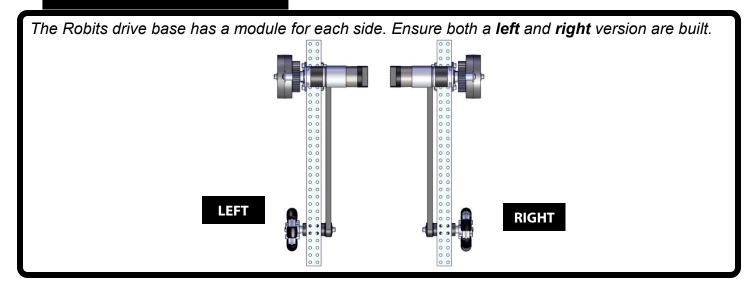
1. Install one 80-100T Motor Mount (am-5017) to the outside of the Robits 1.0 x 1.0 x 15.5 Tube (am-5002-1550) using four 10-32 x 1500 inch screws (am-1014) and four 10-32 nylock nuts (am-1063).
