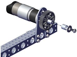
7. Install one 10-32 x 0500 inch screw (am-1002) with one #10 washer (am-1026) into the end of one 4 inch shaft (am-5003-0400).
