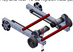
Align the other drive module with the existing inch  $0.5 \times 0.5 \times 10.0$  tubes and fasten with 10-32 x 1750 inch screws (am-1048) and 10-32 Nylock nuts (am-1063).
