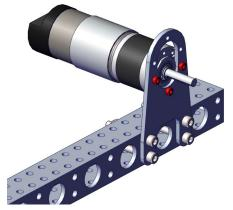
4. Place one 40T gear (am-5020\_40) on the adapter shaft.
