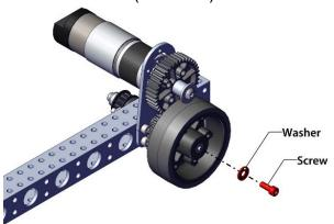
13. Install one 10-32 x 0500 inch screw (am-1002) with one #10 washer (am-1026) into the end of one 3 inch shaft (am-5003-0300).
