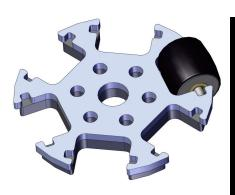
Note: The hub can be used as support under the plates to make it easier to place each of the rollers.
