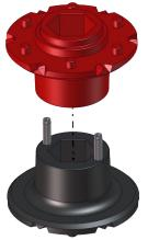
**Step 2:** Press the two 3/32 in. Diameter x 5/8 in. Long Steel Slotted Spring Pins (am-1597) into the two small holes surrounding the hex bore.
