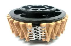
Step 4: Place a #10-32 Nylock Nut on one halve, and tighten its corresponding #10-32 x 1.5" SHCS on the other wheel halve.
