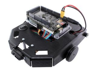
1. Install caster using two Flat Head M3 x 8mm Screws (am-1741) and two M3 Nylock Nuts (am-1023) using the reversible screwdriver. You may have to use pliers to change the screwdriver from a flat head to a phillips head. The flat head of the screw should sit inside the bent flange. The screw and nut can be tightened using the access holes in the frame.
