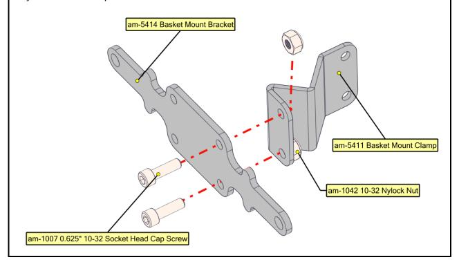
Attach a second Basket Mount Clamp (am-5411) to the assembly created in Step 4 in the same manner. Leave the assembly very loose.
