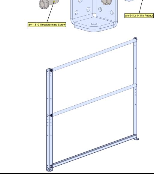
Step 3 Attach (1) am-5416 Left Sheet Metal Outrigger to the frame and (1) am-5415 Right Sheet Metal Outrigger to the frame using (8) 0.5in 10-32 Socket Head Cap Screws (am-1002) and (8) 10-32 Nylock Nuts (am-1042). am-1042 10-32 Nylock Nut am-1002 0.5" 10-32 Socket Head Cap Screw am-5416 Left Sheet Metal Outrigger am-5415 am-5416
