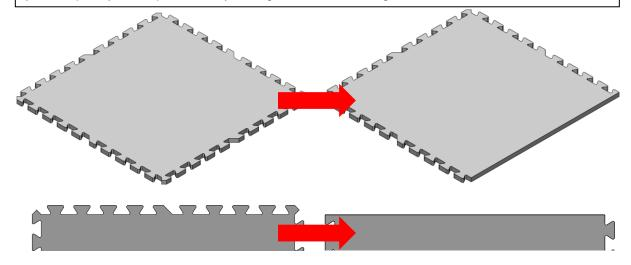
Place the straps centered on the field walls as shown. Use the cut tiles (16 with a single edge cut, 4 with two adjacent edges cut) to form the outer edge of the field floor inside the Field Border. Fill in the rest of the floor with uncut tiles. In total there should be 36 tiles placed.
