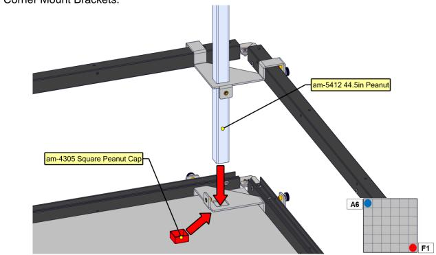
Screw in (2) more #10 Thumb Screws (am-4558) into the Corner Mount Brackets (am-5410). Tighten all six Thumb Screws to secure the entire assembly.
