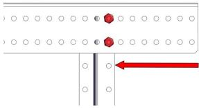
NOTE: The top flange of the Inside Plate should point toward the short side of the End Plate
