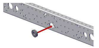
**Step 16:** Secure the Outside Plates to each End Plate using six 10-32 x 0.500 socket head screws (am-1002) and six 10-32 Nylock nuts (am-1042).
