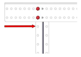
NOTE: The top flange of the Inside Plate should point toward the short side of the End Plate
