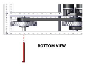
**Step 27:** Repeat steps 19 through 26 to install wheels on other side of chassis.
