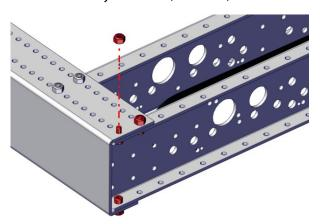
**Step 15:** Place each Outside Plate into the ends of both End Plates with the flanges of the Outside Plate pointing away from the Inside Plate. Ensure the Bearing is aligned to and installed on the ToughBox Mini S Hex Output Shaft.
