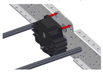
**Step 8:** Attach one ToughBox Mini S to each Inside Plate with four 10-32 x 0.75"SHCS (am-1047) and four 10-32 Nylock nuts (am-1042). The nuts will fit into the hex pockets on the ToughBox Mini S housing and will hold the nut while tightening.
