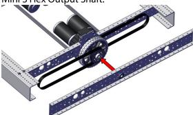
**Step 17:** Attach four 3.375" Churro Standoffs (am-2569) (see below for recommended locations) with 1/4-20 x 0.75" Thread Forming Screws (am-1310) onto each Inside Plate. A 1/2" wrench can be used to hold the churro while tightening. Make sure to loop belts over the churro to ensure the belts have a straight path from axle to axle.
