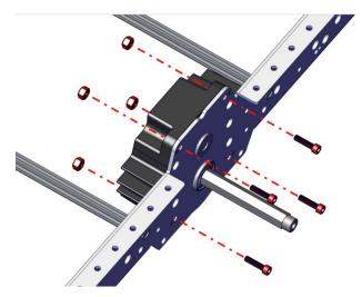
NOTE: Be careful not to overtighten these screws. The gears should spin freely when the shaft is rotated by hand.
