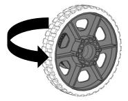
Step 5: Insert one 1/2" Hex Hub (am-2568) into the pulley on one side of the wheel.
