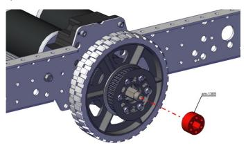
**Step 13:** Select the appropriate belts for your chassis configuration, and loop one belt over each Pulley on each Center Wheel Assembly.
