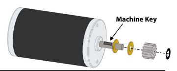
NOTE: Each drive gearbox can accept up to 2 motors. Repeat this step for each motor.
