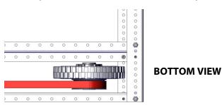
NOTE: The belts should be parallel to the side plates.
