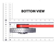
**Step 25:** Slide a %" axle bolt (am-1297) through the spacers and wheel assembly, with the head of the bolt on the outside of the chassis.
