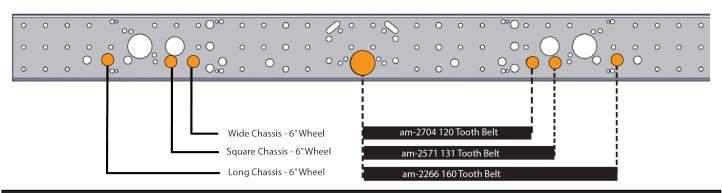
NOTE: Axle bolts must be installed from the outside of the chassis. If they are inserted into the Inside Plate first, the standard bumper hardware will not fit.
