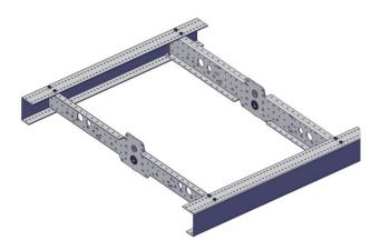
**Step 6:** Attach the two (cut to length) Long Churros between the Inside Plates using four  $\frac{1}{4}$ -20 x 0.750" thread forming screws (am-1310). A  $\frac{1}{2}$ " wrench can be used to hold the churro while tightening.
