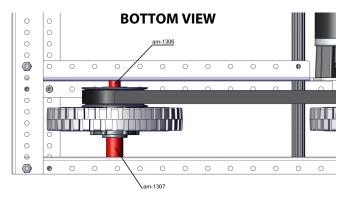
**Step 26:** Install one 3/8-16 Nylock Nut (am-1054) on each Axle Bolt. Tighten the bolt and nut until the spacers just begin to touch Inside and Outside Plates. The wheels should still easily turn, and the axle bolts should be able to spin with a light turn of a wrench.
