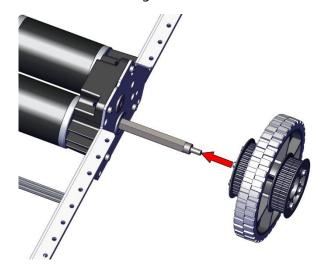
**Step 10:** Line up the CIM motors with the mounting holes in each ToughBox Mini S. Secure each motor with gears installed to the ToughBox Mini S housing using two 10-32 x 0.625" SHCS w/ Nylon Patch (am-1120).
