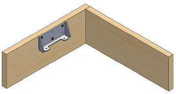
**<u>Step 8</u>**: Once the bracket is in place, install three #8 wood screws (am-1387) into each Side Bracket as shown below.
