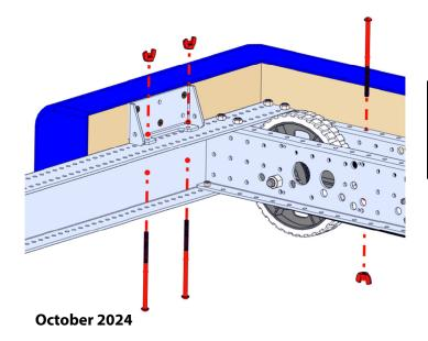
**Note:** On Side Brackets, the wing nuts must be installed on the bottom of the chassis in order to clear the bumper wood. Alternatively, #10-32 nuts can be used.
