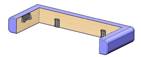
**Step 11:** Attach bumpers as shown with 10-32 x 3.75" round head screws (am-1502) and 10-32 wing nuts (am-1387) for easy installation and removal.
