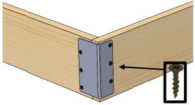
**<u>Step 4</u>**: The Front Bracket (am-3961) is designed to be a robust attachment for the bumper onto the AM14U End Plate. The holes on the bottom bracket will align with holes on the End Plate and can be placed anywhere along the frame to avoid hardware or mechanisms.
