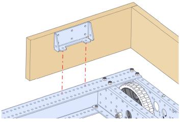
**<u>Step 5</u>**: Line up the top edge of the Front Bracket with the top edge of the plank assembly.
