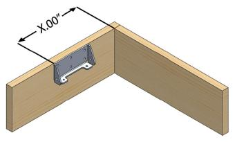
**Step 7:** The Side Bracket (am-3962) will need to fit between the flanges on the Outer Plate of the AM14U6. To align with the holes, the edge of the bracket should be an integer number of inches away from the inside corner.
